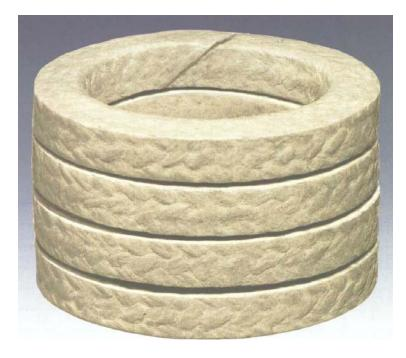
RAMILON is braided from Ramie, an extremely strong and water-resistant natural fibre. The packing also contains a high level of PTFE due to a comprehensive impregnation process. This ensures high density and low friction performance. RAMILON is also widely used in plunger pumps for high-pressure water applications.
